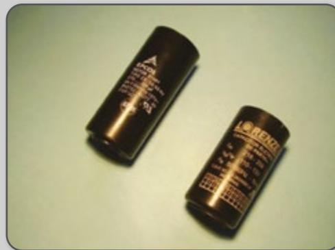
**2** Capacitores eletrolíticos.
