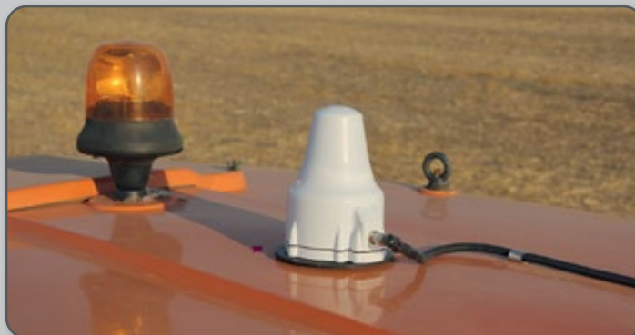
Figura 28 – Receptor GNSS instalado no trator.
