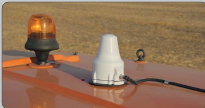
Figura 28 – Receptor GNSS instalado no trator.
